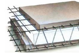
Truss Reinforced Insulated Concrete Eco-Wall developed by Braj Green Product , India
